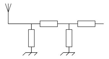
Each element could be an inductor or a capacitor. A DC path from antenna to ground is strongly recommended for ESD avoidance.
