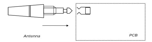
Antenna is screwed on chassis. Metallic part of the antenna support a M4x0,5 screw.
