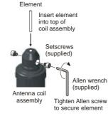
Note: Installation of the **ATAS-120** on a hatchback or trunk lid may not permit a low SWR to be obtained. A solid bond to the car body is important so as to establish a counterpoise for the vertical radiating element.
